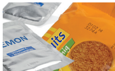
Flexible packaging – colour change, top layer removal
